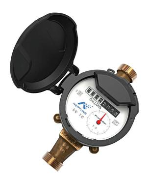
The Neptune® ProCoder™ solid state absolute encoder register features a high-resolution, mechanical sweep hand to detect ultra-low flows as well as monitor direction of flow. The ProCoder's non-contact LED absolute encoding technology ensures the odometer read exactly matches the remote read. It provides a high-resolution, 8-digit remote meter reading along with leak, tamper, and reverse flow flags when connected to a Neptune R900® MIU.
